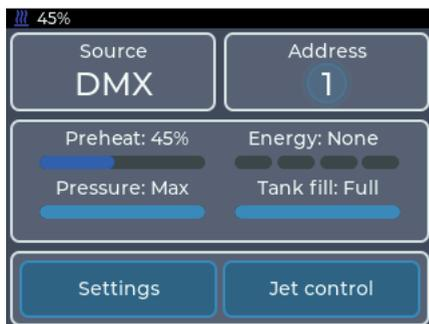
Fig. 1: Main menu - OctaJet when heating up
