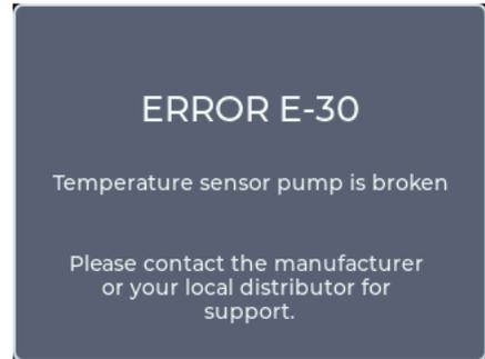
The temperature sensor inside the pump is defective/broken.
